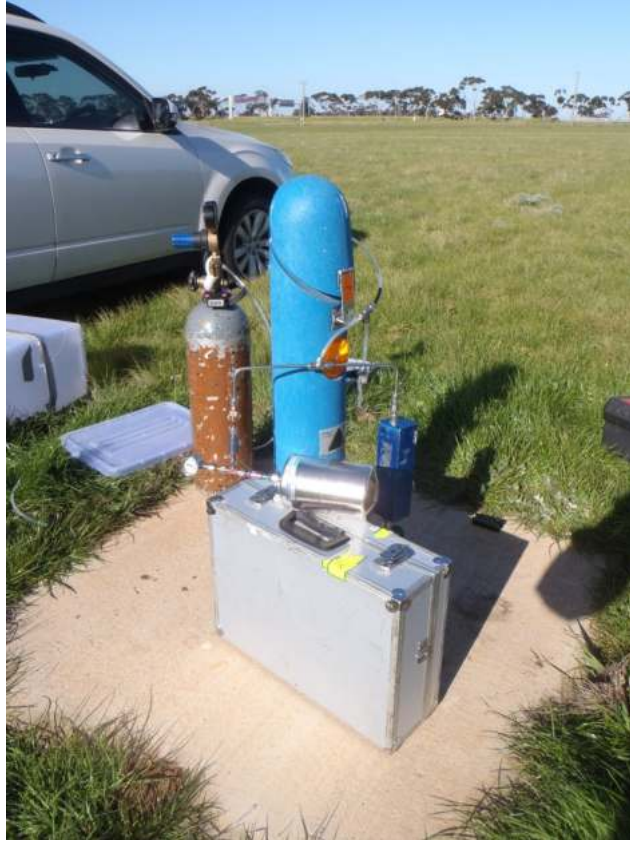
Figure 4-1: Soil Vapour Sampling (Primary Sample and Auditor Verification Sample)
