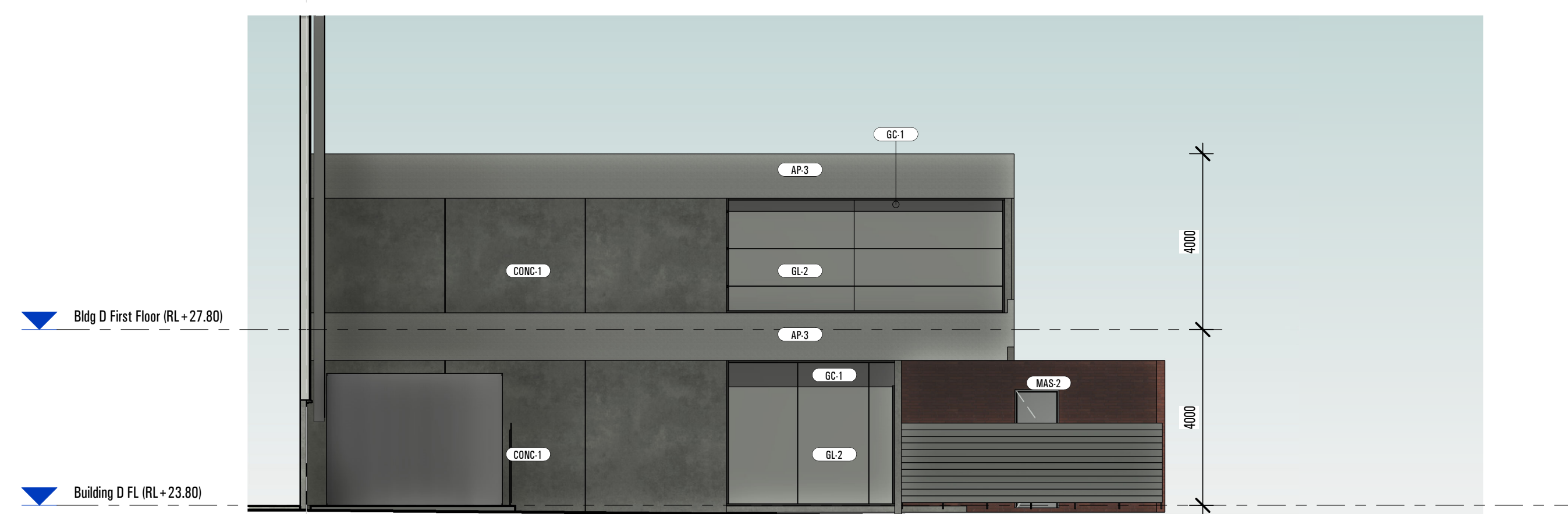
N Bldg D Office - North Elevation 1 : 100
